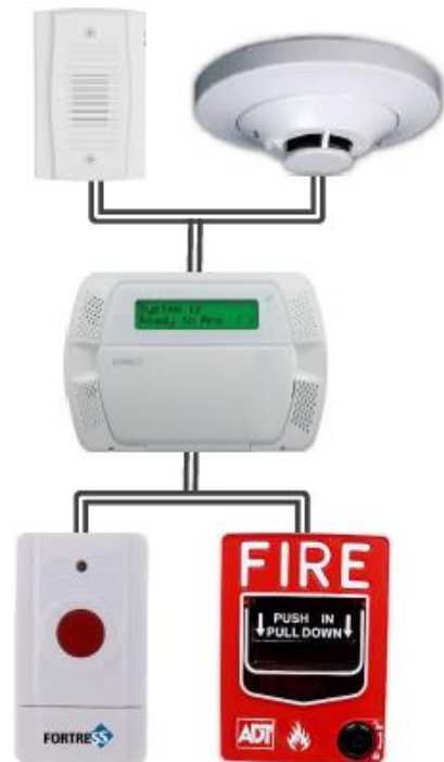
Combination fire & burglar alarm system with pull station or panic button activating smoke alarms and/or mini-horns
